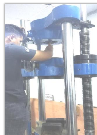
Fig.9 - Tensile test on UTM (TUTE 60 T) Machine
